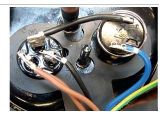
5 Ensure that the insulation is placed as shown here. If not, insulate as shown.
