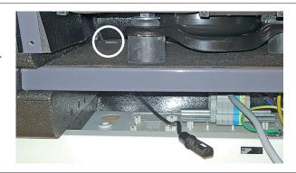
**10.** Find the compressor compartment cover with the pre-mounted bracket for the humidity sensor.
