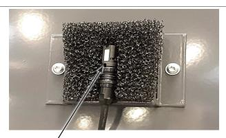
Note: the white surface and hole in the sensor must be facing front.
