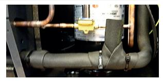
Ensure that the wire for the solenoid valve is not close to the compressor.
