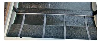
The new PPI filter must be right up against both ends of the cabinet.
